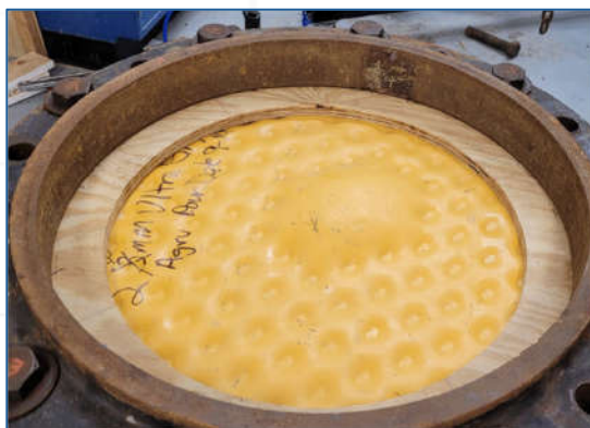
Figure 3: Liner Hydraulic Pullout Resistance Test
