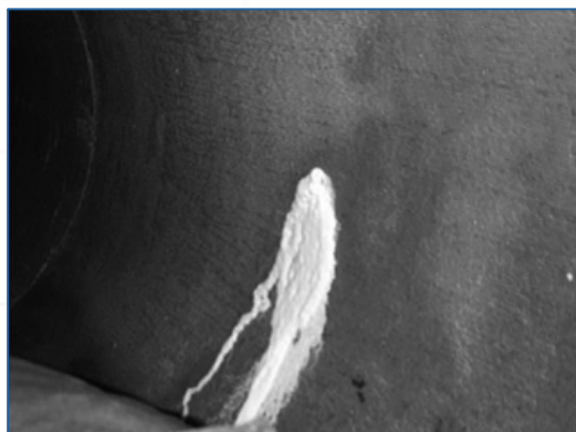
Figure 1: Autogenous Healing from Pinhole
