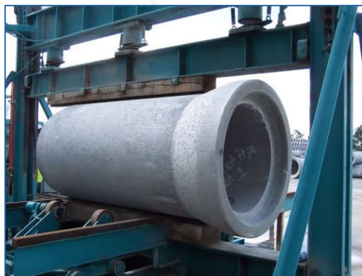
Figure 2: Three Edge Bearing (3EB) Testing Assembly
