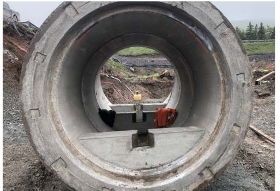
2946mm ID concrete pipe with a 3775mm OD special design 829mm wall thickness, 135 lineal meters, 56 pipe sections with slopes and fish weirs
