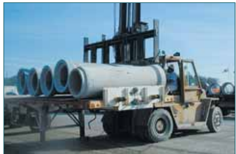
Shipping Concrete Pipe
