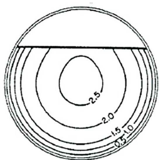
*Typical Curve of Equal Velocity Relative to Mean Velocity in a Pipe*
