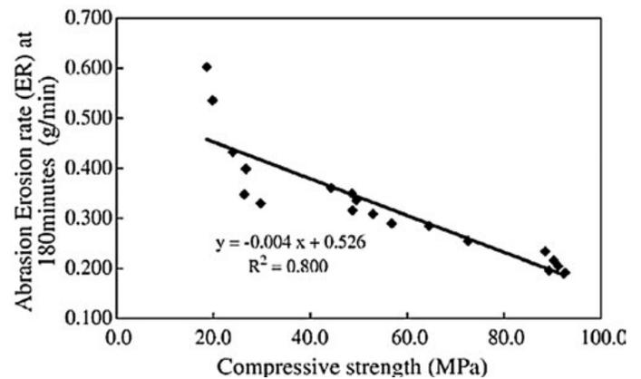
Figure 2: The relationship of compressive strength and abrasion erosion rate
