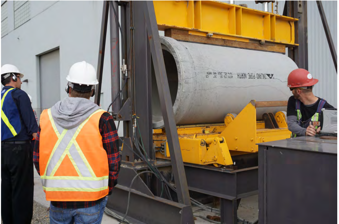
Ultimate strength three-edge bearing test of Class III, 300 mm reinforced concrete pipe. Photo by Inland Pipe
